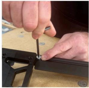
SLIDE THIS UP TO THE RAIL SQUARE AND USING T HE 3MM HEX KEY TIGHTEN THIS UP AND THAT IS N OW CALIBRATED.
