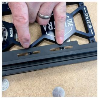
LINE UP THE REPEAT STOP SLOTS TO THE RS H OLES ON THE RAIL SQUARE
