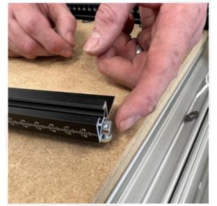
THEN SLIDE THE CALIBRATION SCREW WITH THE ATTACHED T-NUT INTO THE REPEAT STOP ON THE UNDERSIDE.
