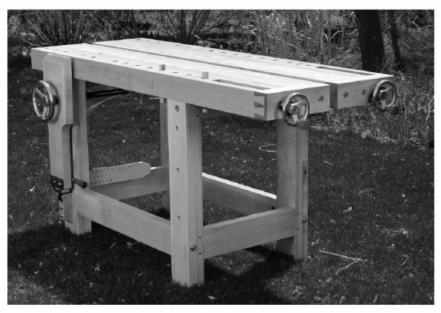
We then built a larger, 87" long version of the Split-Top Roubo with a more robust base with legs at 5-3/8" x 3-1/2", modeled after Roubo's original 6" x 3" legs, a sliding dead-man, shelf, and a new accessory, the "Gap Stop", to further take advantage of the gap be-tween the tops.
