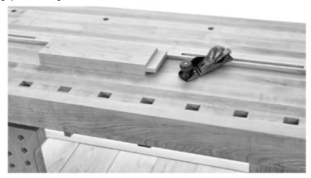
We've designed the base with knockdown joints on the long rails using our own knockdown hardware: Bench-
