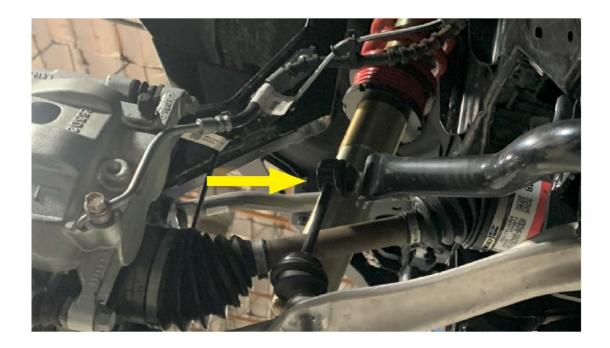
Remove the pivot bushing bracket bolts holding the sway bar assembly in place. Detach the sway bar from the vehicle.
