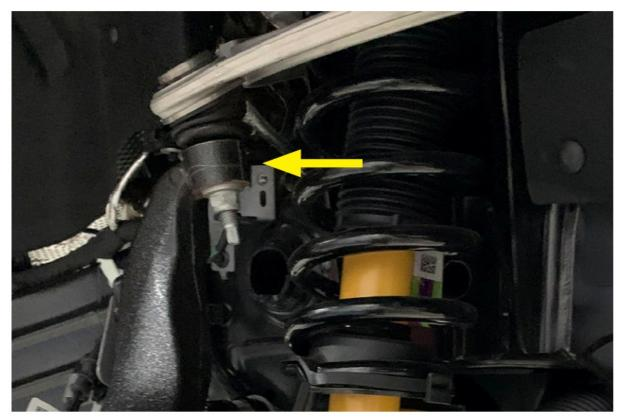
14. Using 21mm and 24mm wrenches, remove the upper arm bolt and nut to detach the control arm from the vehicle.
