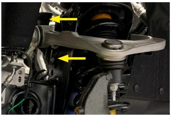
11. Locate the steering linkage on the driver side. Use a paint pen mark a line on the both the U-joint and at the firewall. Remove the bolt from the coupler and slide the linkage away. Do not allow the upper and lower shafts to rotate.
