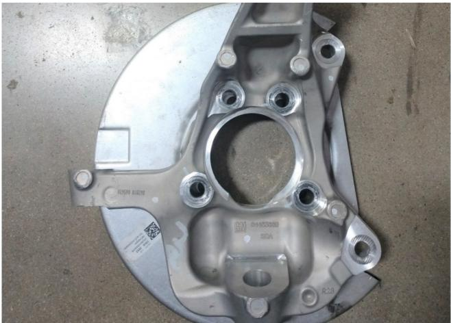
17. Remove the two O-rings from the original knuckle and place them on the new Belltech spindle. Attach the hub assembly and bearing shield on the Belltech spindle, torque the hub bolts to 111 ft lbs. + 30-45 degree turn.
