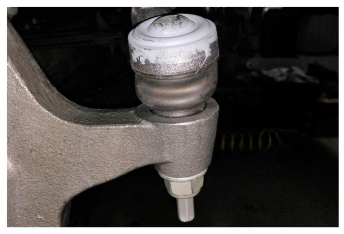
14. Loosen the lower ball joint nut for the ball joint removal using a 24mm socket. It may be helpful to use an hex
