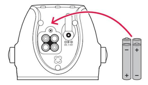
Warning! ONLY USE RECHARGEABLE NIMH BATTERIES. Non-rechargeable batteries will start to leak and the battery acid will damage the electronics. The resulting damage is not covered by warranty.
