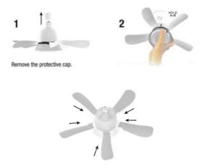
I needed, use the socket extender. Screw it in clockwise. Do not overtighten, but make sure the fan is fully secured. Then, follow step 2 to install the Socket Fanlight unit.
