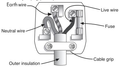
The wires in the mains lead are coloured in accordance with the following code: Blue Neutral (N) Brown Live (L)
