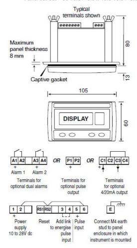
Abbreviated instructions for BA367E-SS Rugged one input intrinsically safe Counter
