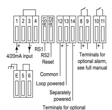
Terminals 2 & 4 internally linked for joining return 4/20mA wire.
