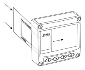
To replace the scale card carefully insert it into the slot shown in Fig 2. Force should be applied evenly to both sides of the scale card to prevent it twisting. The card should be inserted until about 2mm of the transparent tab remains protruding.
