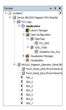
I/O Modules can be added under the BA3101 Pageant Operator Panel device, right click on any of the 7 slots corresponding to the slots on the rear panel of the BA3101 Display and select Plug Device. A list of all the I/O modules available will appear, select the Module required for the application and click on Plug Device.
