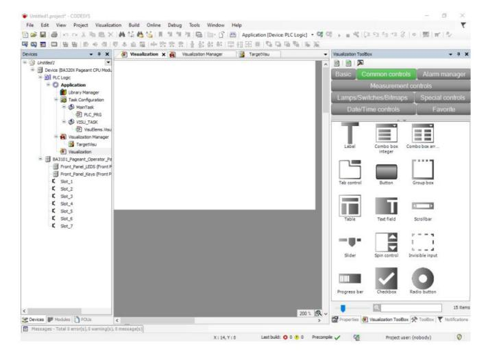
The screen sizes is already set up to 320 X 240 pixels to match with the LCD size of the Display and the fonts are restricted to the list of fonts available in the BA3101 Display.
