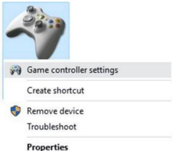
3. Click "properties" to open the interface for testing the keys. Use the "X axis/Y axis" to test the left stick, the "Z axis" to test the LT/RT key, the "X rotation/Y rotation" to test the right stick, the "Keys" to test each function key, and the "Point of View Hat" to test the cross key.
