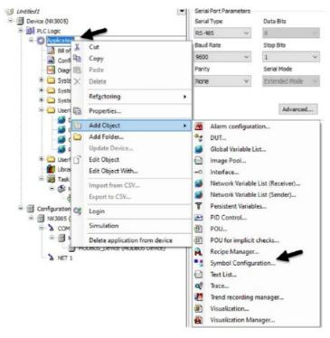
2. In the new window, click on Add and then on Build in the Symbol Configuration section.
