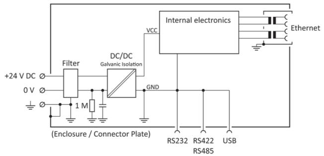
The HMI panel has galvanic isolation against the 24 V DC power supply but no galvanic isolation between the communication ports for RS-232, RS-422, RS-485 and USB. Only the Ethernet connection has galvanic isolation.
