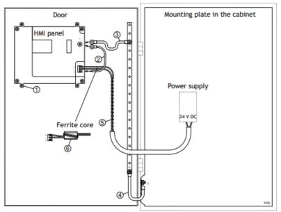
The mounting clamps of the HMI panel do not provide a secure grounding connection between the panel and the device cabinet, see 1 in drawing above. To ground the HMI panel:
