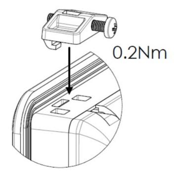
Tighten the screws to 0.15 - 0.2 Nm.
