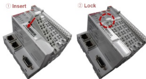
Mount a removable terminal block
