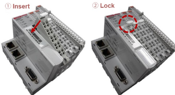
Mount a removable terminal block
