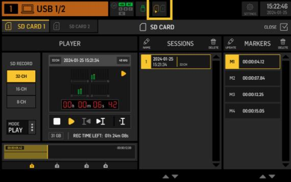
Up to 64 channels can be recorded on two SD cards in the WING-LIVE expansion card. 32 channels will be
