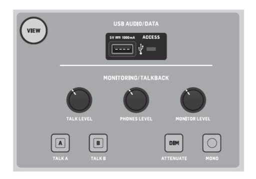
A USB type-A connector allows a flash drive to be plugged directly into the console for saving or loading data. This allows you to always have a backup of your show files, or even use a rented WING console while retaining your usual setup.
