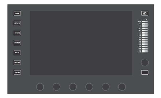
The majority of the WING's controls can be edited and monitored via the 10" touch screen Main Display. Various screens can be accessed with the 7 buttons along the left side of the screen, as well as the VIEW buttons located in each major section of the top panel.
