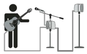
Set all controls as shown: HIGH, MID and LOW knobs to their centered position at 12 o'clock;
