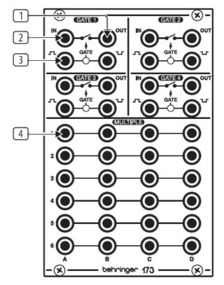
GATE OUT - Send the gate signal to another module via 3.5 mm TS cable.
