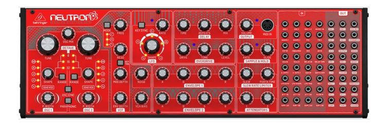
Paraphonic Analog and Semi-Modular Synthesizer with Dual 3340 VCOs, Multi-Mode VCF, 2 ADSRs, BBD Delay and Overdrive Circuit in a Eurorack Format
