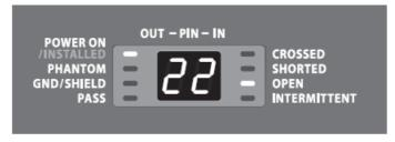
• When testing an XLR cable, if the display shows this combination, it indicates there is a short between pin 1 and pin 2. This short may be on the "in" side or the "out" side.
