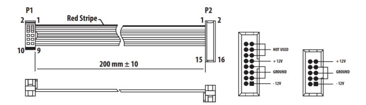
The module comes with the required power cable for connecting to a standard Eurorack power supply system. Follow these steps to connect power to the module. It is easier to make these connections before the module has been mounted into a rack case.
