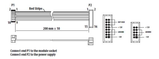
The CM1A module comes with the required power cable for connecting to a standard Eurorack power supply system. Follow these steps to connect power to the module. It is easier to make these connections before the module has been mounted into a rack case.
