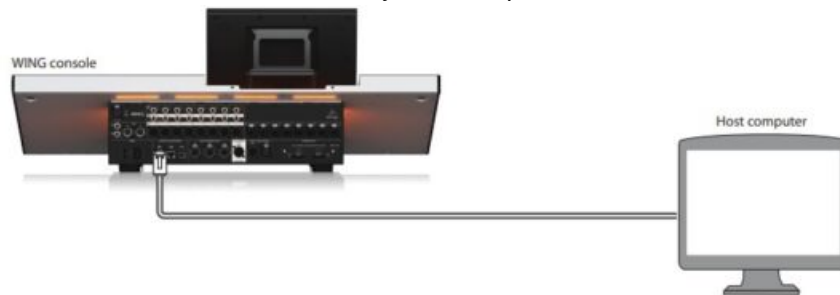
Fig. 1: Direct connection between WING and host computer
