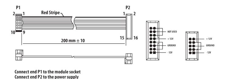
The module comes with the required power cable for connecting to a standard Eurorack power supply system. Follow these steps to connect power to the module. It is easier to make these connections before the module has been mounted into a rack case.
