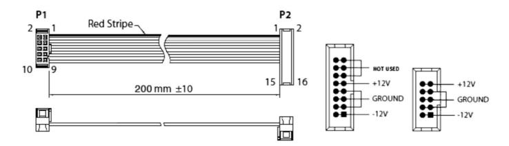
The 961 INTERFACE module comes with the required power cable for connecting to a standard Eurorack power supply system. Follow these steps to connect power to the module. It is easier to make these connections before the module has been mounted into a rack case.
