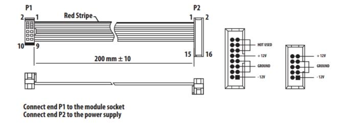
The 182 SEQUENCER module comes with the required power cable for connecting to a standard Eurorack power supply system. Follow these steps to connect power to the module. It is easier to make these connections before the module has been mounted into a rack case.
