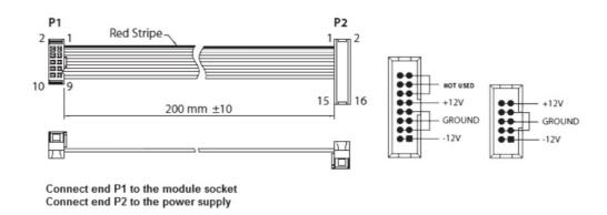
The unit comes with the required power cable for connecting to a standard Eurorack power supply system. Follow these steps to connect power to the module. It is easier to make these connections before the module has been mounted into a rack case.
