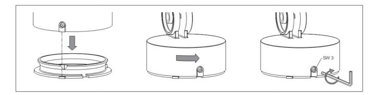
Place the floodlight unit onto the mounting plate as displayed in the sketch, and align and screw it together firmly.
