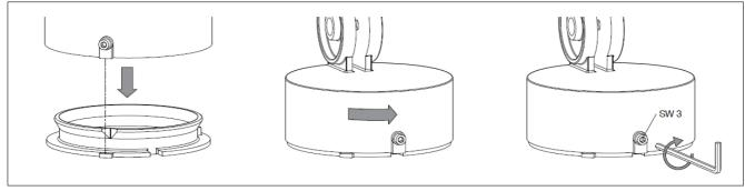
• Place the floodlight unit onto the mounting plate as displayed in the sketch, and align and screw together firmly.
