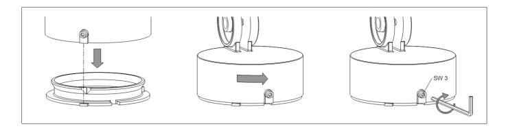
Place floodlight unit onto the mounting plate as displayed in the sketch, align and screw together firmly. Adjustment of beam direction:
