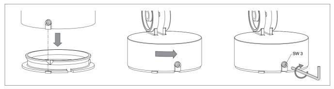
Place floodlight unit onto the mounting plate as displayed in the sketch, align and screw together firmly.
