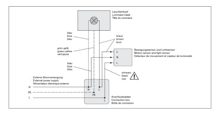
Close the connection box. Lead the bollard tube on the anchorage unit and align. Tighten the screws evenly. Screw the glass with the gasket into the luminaire housing and tighten firmly. Make sure that the glass gasket is seated correctly (see sketch).
