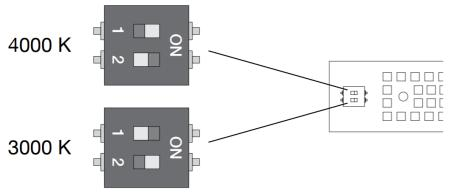
The colour temperature of the LED module was set to 3000 K by default (switch position 2: "on", 1: "off"). For colour temperature 4000K, the switch position 2: "on" and 1: "off" must be selected.
