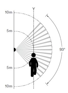
The specifications for the range and detection area of the PIR motion sensor are reference values. The detection area is up to 110° horizontally and 93° vertically, with a depth of max. 10 m depending on the direction of motion (see sketch). Too minor temperature difference between the moving object and the ambient temperature can influence the detection range. Local conditions and external heat sources may affect both the range and the detection area.
