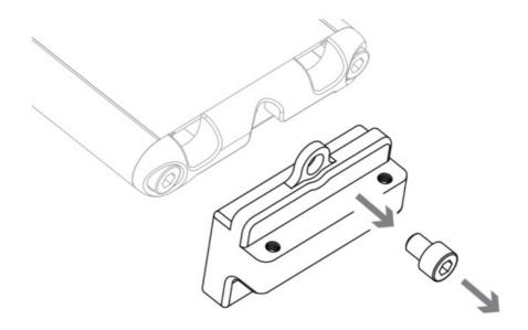
3.2 Place the adapter into the rear frame of Tenon.
