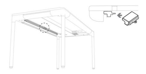
3.3 Lower Basalt through the desktop slot onto the adapter from above.
