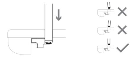
3.4 Fasten the middle bolt to secure both parts together.
