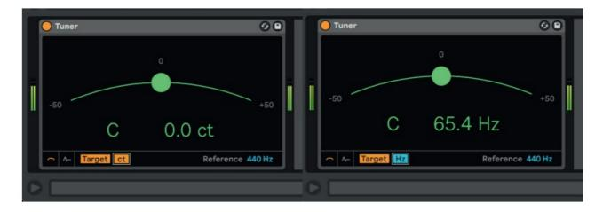
5. Move up the Octave switch to the fifth position (marked with 0 on the front panel) and check the Tuner. The note should be close to C5. Adjust the V/Oct trim-pot carefully till you get C5 and 0 cents.
