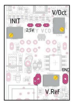
2. Pick your multimeter and select DC Voltage mode (typically marked as V=). Connect the black probe to a Ground point (you can use the sleeve of patch cable connected to any other module) and place the red probe touching the point marked.
