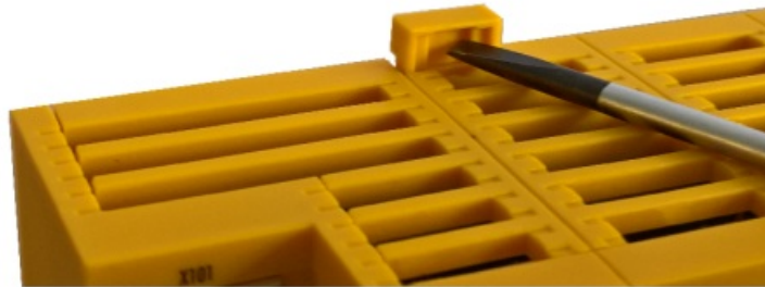
Fig. 20: DIN rail clamp opened
