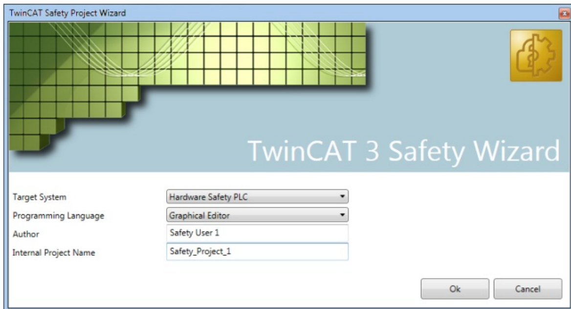
Fig. 26: TwinCAT Safety Project Wizard
