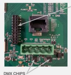
To replace, solder the DMX chips to the 8 pin connectors.
