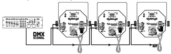
CAUTION! At the last unit, you must close the DMX line with a terminating resistor. Take an XLR connector and solder a 120 Ohm resistor between signal (-) and signal (+) and connect it to the DMX output of the last unit in
