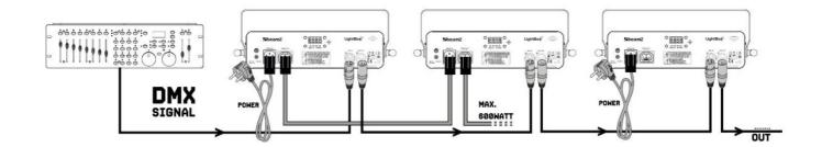
CAUTION!At the last unit, you must close the DMX line with a terminating resistor. Take an XLR connector and solder a 120 Ohm resistor between signal (-) and signal (+) and connect it to the DMX output of the last unit in the line.
