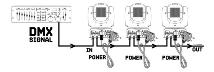
**CAUTION:** At the last unit, you must close the DMX line with a terminating resistor. Take an XLR connector and solder a 120 Ohm resistor between signal (-) and signal (+) and connect it to the DMX output of the last unit in the line.
