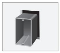
When installing jamb version, cutout dimensions are 1 ½" (W) x 2 ¾" (H) × 1" (D min)
