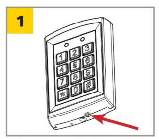
Using the supplied hex key, remove the backcase screw from the keypad bottom.
