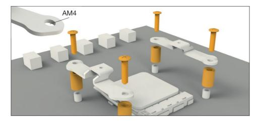
Place the four AMD spacer nuts (9) over the bolt threads of the backplate on the front side and fix both the AMD mounting brackets (6) using the AMD backplate screws (12).
