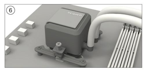
Place the CPU block centrally over the Intel mounting brackets (4) or Intel mounting brackets LGA 1700 (5), such that these allow the CPU block to be screwed down. For this you can use a normal crosshead screwdriver. Next connect the pump to the motherboard.
