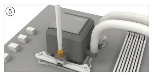
Place the CPU block centrally over the Intel mounting brackets (4), such that these allow the CPU block to be screwed down. For this you can use a normal crosshead screwdriver. Next connect the pump to the motherboard.
