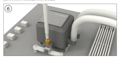
Place the CPU block centrally over the short AMD mounting brackets (6), such that these allow the CPU block to be screwed down. For this you can use a normal crosshead
