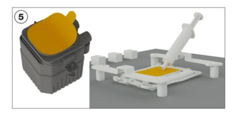
Place the CPU block centrally over the Intel mounting brackets, such that these allow the CPU block to be screwed down. For this you can use a normal crosshead screwdriver.
