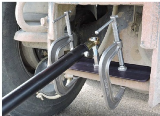
Figure 8: Appropriate Ball Joint Positioning
