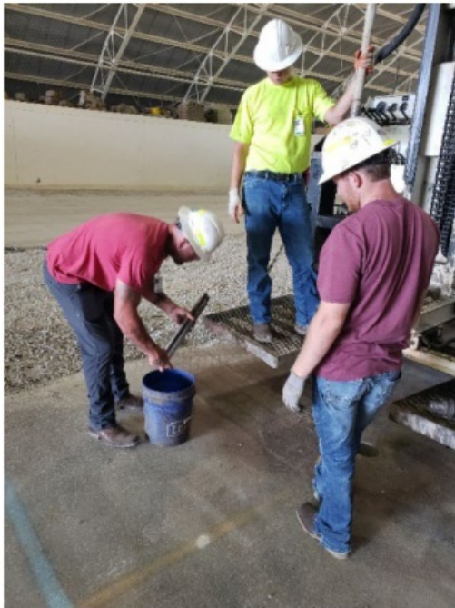
Figure 7: Left- operators cleaning the dirt from the split spoon, Right- operators putting the split spoon back onto the rig in preparation for another plunge
