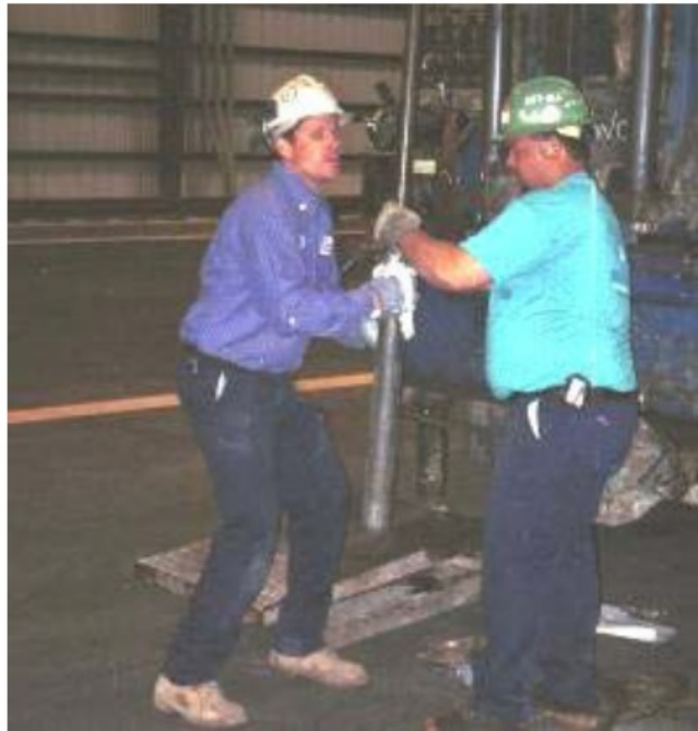
Figure 7: Left- operators cleaning the dirt from the split spoon, Right- operators putting the split spoon back onto the rig in preparation for another plunge
