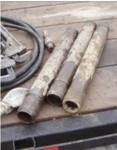
Figure 6: Split spoon heads used to create the borehole for the MDD
