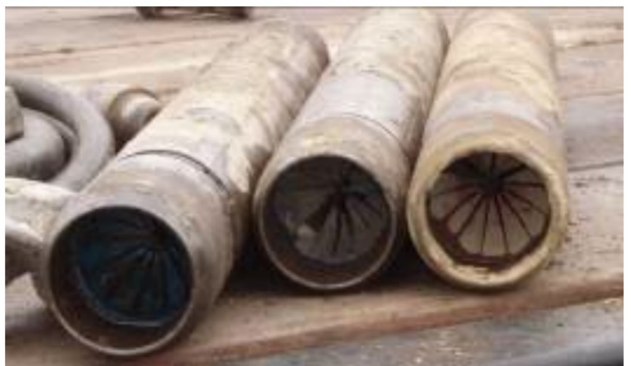
Figure 6: Split spoon heads used to create the borehole for the MDD
