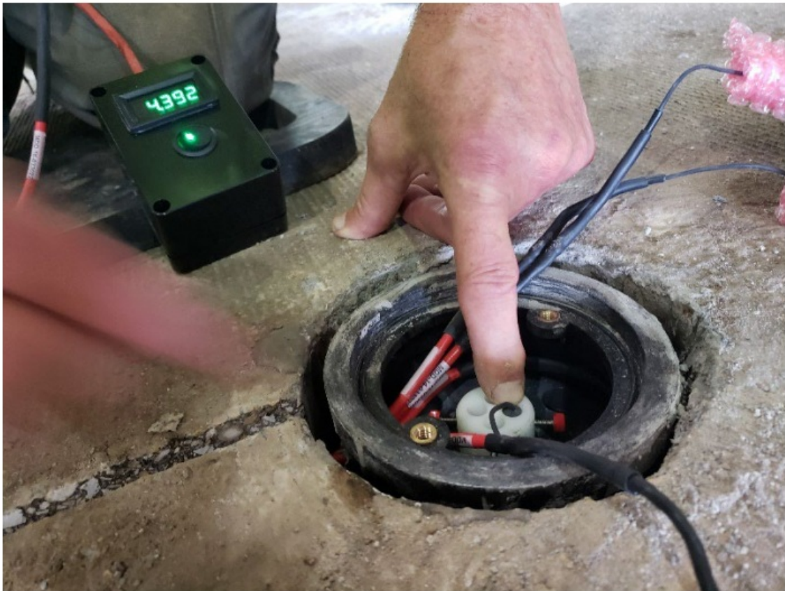
Figure 16: Sensor being installed into the sensor cavity, using the readout box to ensure that it is installed in a very slightly compressed position
