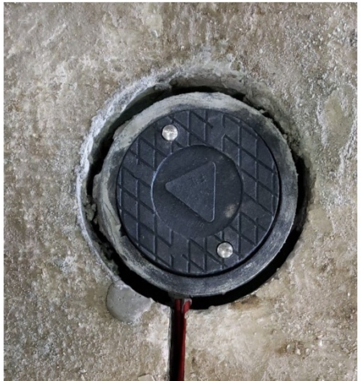
Figure 16: Sensor being installed into the sensor cavity, using the readout box to ensure that it is installed in a very slightly compressed position
