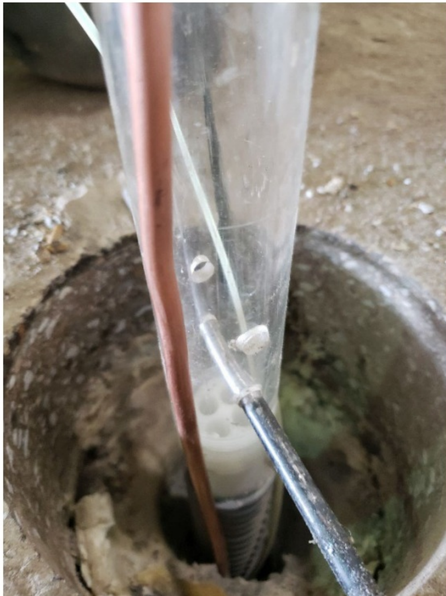
Figure 10: Connecting rod inserted into the setting tube, through the bottom set of holes (this example excludes the threaded rods in each measurement position)
