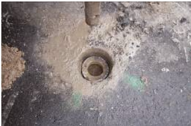
Figure 8: Wooden doughnut being used to guide the split spoon through the center of the corehole
